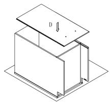
Step 5 : Install screw(5) Ø3.5x35mm
