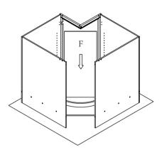
Step 9 : Install screws of back panel (F) and big side panels(C) with (5)  $\not\! o 3.5x35mm$  screws.
