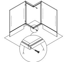
Step 4: Insert the bottom panel(D) into the side
