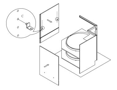
Step 8: Install the back panel(F). Insert the back panel into the two big side panels.
