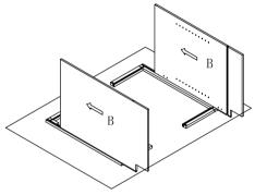
Step 3: Install screws of front frame with (4) \( \varphi 3.5x35mm \) screw.
