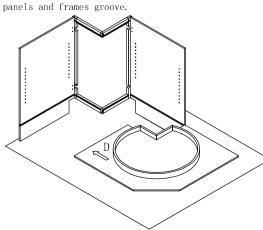
Step 5 : Install shelf clips. Install the shelf clips to small side panels.
