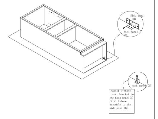
Step 8: Install door panel(J) and corner block screw the hing to the door and face frame, then install rainbow bracket to the side panel (B), front frame (A) and back panel (D) with the (4)  $\emptyset$ 3.5x16mm screw.
