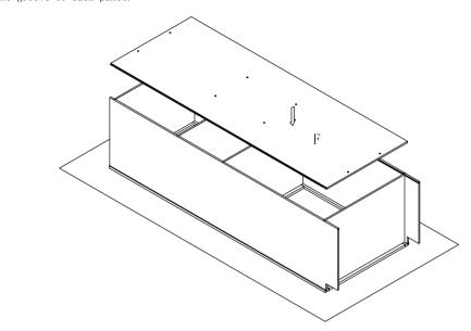
Step 5 : Install assembly screws (5)  $\emptyset$ 3.5x35mm into back panel (D) then fit in the L-shape insert bracket from front frame (A) into bottom panel (C) bracket and screw the bracket with (3)  $\emptyset$ 3.5x14mm screw
