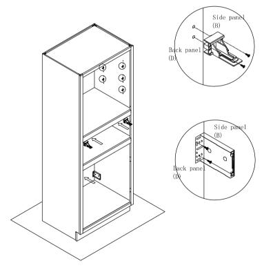
Step 10: Install adjustable shelf(H) and drawer slide. Put the adjustable shelf on the shelf clips and Insert drawer slide runner to the rear slide bracket and screw the drawer slide to the guide hole of front frame (A) and hole for drawer slide, then screw the steel ball slide to the drawer side panel of drawer box.
