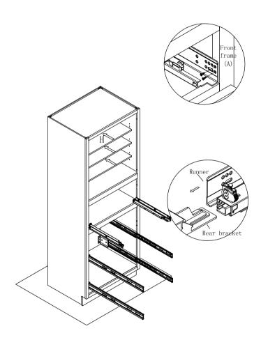
Step 11: Put the drawer box on the drawer slide and push the drawer box to make it the end of the runner is locked to the hole of the drawer back panel. Complete the installion of the drawer box when you hear the sound "click" which means the locking device is locked on the drawer slide.
