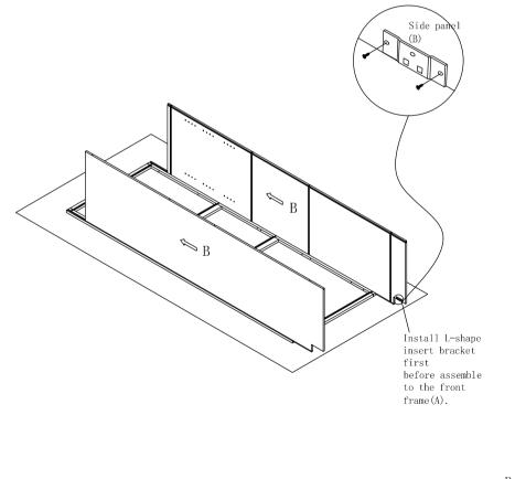
Step 3 : Install top&bottom panel and fixed shelf. Insert top panel(D) bottom panel(C) and fixed shelf (E) into groove of front frame (A) until it into the groove of front frame (A).
