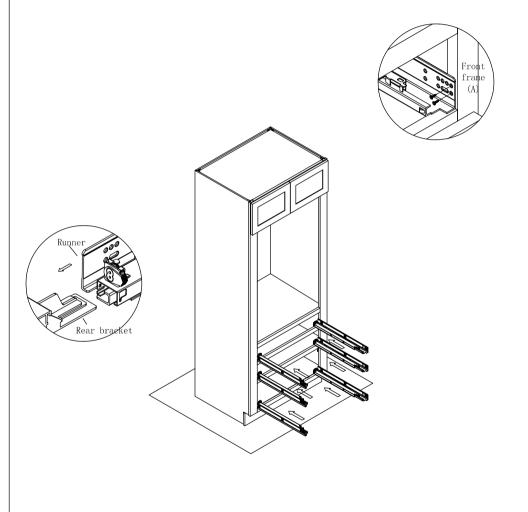
Step 11: Put the drawer box on the drawer slide and push the drawer box to make it the end of the runner is locked to the hole of the drawer back panel. Complete the installion of the drawer box when you hear the sound "click" which means the locking device is locked on the drawer slide.
