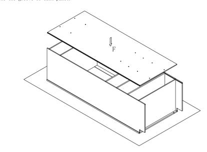
Step 5: Install assembly screws (5)  $\emptyset$ 3.5x35mm into back panel (D) then fit in the L-shape insert bracket from front frame (A) into bottom panel (C) bracket and screw the bracket with (3)  $\emptyset$ 3.5x14mm screw
