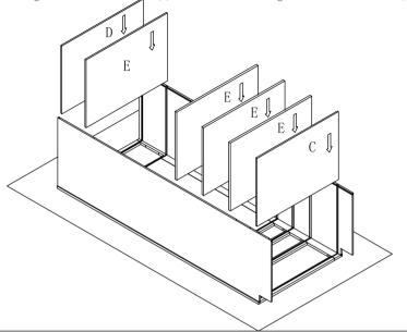
Step 4: Install back panel(F).until bottom panel and top panel and fixed shelf into the groove of back panel.
