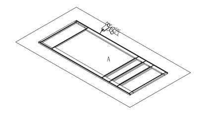
Step 2: Install side panels. Insert side panel into groove of front frame (A) until side panel and front frame even.
