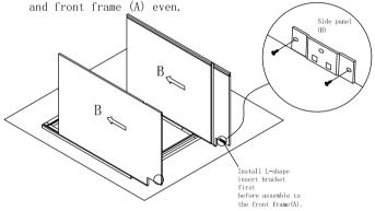
Step 3: Install bottom panel. Insert the bottom panel (C) into groove of side panel (B) until it into the groove of front frame(A).
