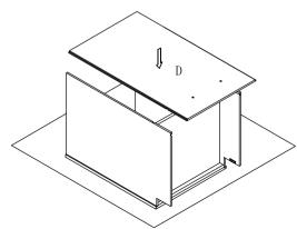
Step 5 : Install screw(5) Ø3.5x35mm
