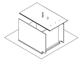
Step 5 : Install screw(5) Ø3.5x35mm
