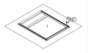
Step 2: Install side panel. Insert both side panel (B) into groove of front frame (A) until side panel (B)
