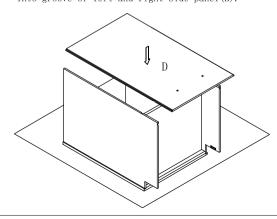
Step 5 : Install screw(5) Ø3.5x35mm
