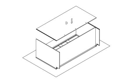
Step 5 : Install screw(5) \( \phi 3.5 x 35 mm \) into back panel (D).
