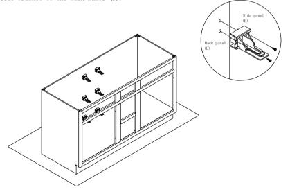
Step 10: Insert drawer slide runner to the rear slide bracket and screw the drawer slide to the guide hole of front frame (A) and hole for drawer slide
