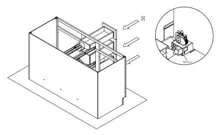
Step 12: Install door panel (G). Screw the hinge to the front frame (A) and door (G).
