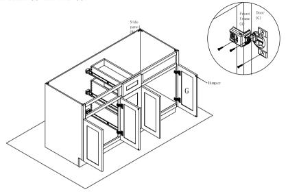
Step 13: Screw wood connect on the front frame.
