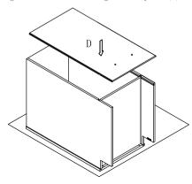
Step 5 : Install screw(5) Ø3.5x35mm
