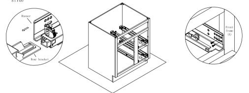
Step 11: Put the drawer box on the drawer slide and push the drawer box to make the end of runner is lock to the hole of the drawer back panel. Complete the installation of the drawer box when your hear sound click which mean the locking device is locked on the drawer slide.
