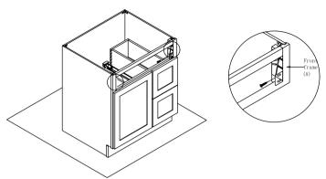
Step 15: Install drawer front ,then install the overhead door hinge box to the drawer front.
