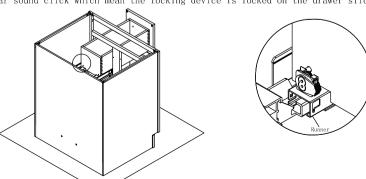
Step 12: Install door panel (G). Screw the hinge to
