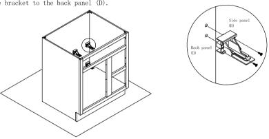
Step 10: Insert drawer slide runner to the rear slide bracket and screw the drawer slide to the guide hole of front frame (A) and hole for drawer slide
