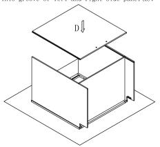
Step 5 : Install screw(5) Ø3.5x35mm into back panel (D).
