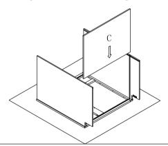
Step 4: Install back panel. Insert back panel (D) into groove of left and right side panel(B).
