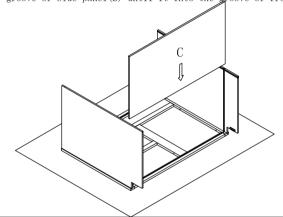
Step 6: Install toe kick panel. Fit in the L-shape insert bracket from toe kick panel (E) into side panel (B) bracket and screw the bracket with(3) Ø3.5x14mm
