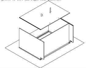
Step 2: Install side panel. Insert both side panel(B) into groove of front frame(A) until side panel(B) and front frame(A) even.
