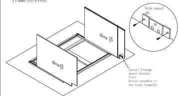
Step 5 : Install screw(5) Ø3.5x35mm
