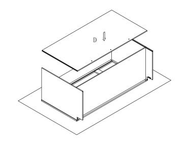
Step 5 : Install screw(5) \( \phi 3.5 x 35 mm \) into back panel (D).
