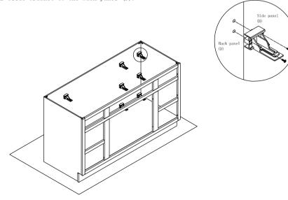
Step 10: Insert drawer slide runner to the rear slide bracket and screw the drawer slide to the guide hole of front frame (A) and hole for drawer slide
