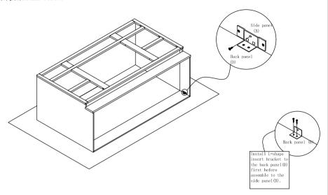
Step 8: Install corner block. Install rainbow bracket to the side panel (B), front frame (A) and back panel (B) with the (4) \$\phi\_3.5x16mm\$ screw.
