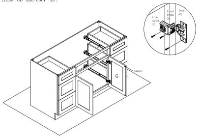
Step 13: Screw wood connect on the front frame.
