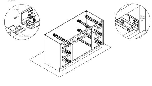
Step 11: Put the drawer box on the drawer slide and push the drawer box to make the end of runner is lock to the hole of the drawer back panel. Complete the installation of the drawer box when your hear sound click which mean the locking device is locked on the drawer slide.
