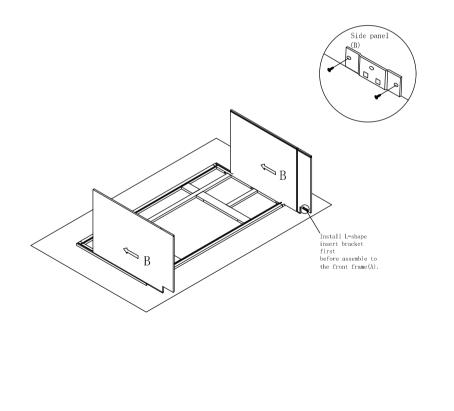
Step 3: Install bottom panel. Insert the bottom panel (C) into groove of side panel(B) until it into the groove of front frame(A).
