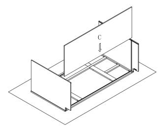
Step 4: Install back panel. Insert back panel (D) into groove of left and right side panel(B).
