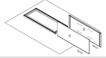
Step 3: Install top and bottom panel. Insert top and bottom panel (C) into groove of side panel (B) until it into the groove of front frame (A).
