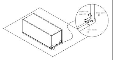
Step 6: Install screw(5) \( \varphi 3.5x35mm \) into back panel (D), then nails side panel(B) and back panel(C) using
