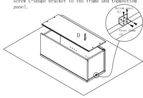
Step 5 : Screw rainbow bracket into front frame(A) and side panel(B).
