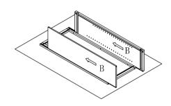
Step 3: Install top and bottom panel. Insert top and bottom panel (C) into groove of side panel (B) until it into the groove of front frame (A).
