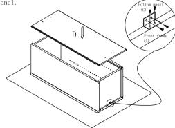
Step 5 : Screw rainbow bracket into front frame(A) and side panel(B).
