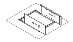
Step 3: Install top and bottom panel. Insert top and bottom panel (C) into groove of side panel (B) until it into the groove of front frame (A).
