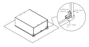
Step 6 : Install screw(5)  $\emptyset$ 3.5x35mm into back panel (D), then nails side panel(B) and back panel(C) using
