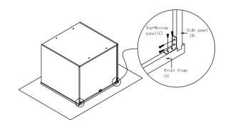
Step 6: Install screw(5) \( \varphi 3.5 x 35 mm \) into back panel (D), then nails side panel(B) and back panel(C) using
