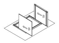
Step 3: Install top and bottom panel. Insert top and bottom panel (C) into groove of side panel (B) until it into the groove of front frame (A).
