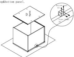
Step 5: Screw rainbow bracket into front frame(A) and side panel(B).
