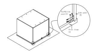
Step 6 : Install screw(5)  $\mbox{\it Ø3.5x35mm}$  into back panel (D),then nails side panel(B) and back panel(C) using
