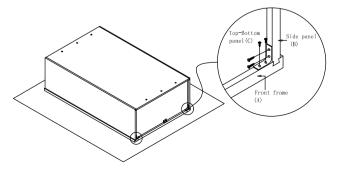
Step 6: Install screw(5) \( \varphi 3.5 x 35 mm \) into back panel (D), then nails side panel(B) and back panel(C) using
