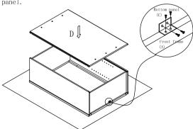
Step 5 : Screw rainbow bracket into front frame(A) and side panel(B).
