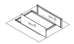
Step 3: Install top and bottom panel. Insert top and bottom panel (C) into groove of side panel (B) until it into the groove of front frame (A).
