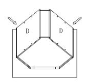
Step 5: Install the back panel.
