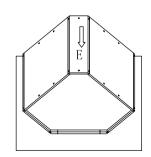
Step 6 : Screw the big side panels and top&bottom panel ,also screw the back panel and top\*bottom panel.
