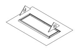
Step 3: Install small side panel. Insert small side panel (C) into groove of front frame (A) until it into the groove of front frame (A).
