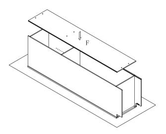
Step 5: Install assembly screws(5) \( \phi 3.5 x 35 mm \) into back panel (D).
