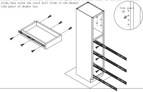
Step 10: Install adjustable shelf(H) and drawer box(I). Put the adjustable shelf on the shelf clips and insert the drawer slide of drawer box to the drawer slide of side panels.
