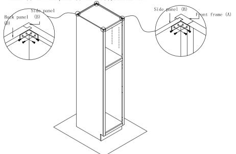
Step 9: Install shelf clips and steel ball slide. Insert shelf clips into the side panels, then Screw the rear slide bracket to the back panel (F). Insert drawer slide runner to the rear slide bracket and screw the drawer slide to the guide hole of front frame (A) and hole for drawer slide, then screw the steel ball slide to the drawer
