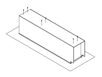
Step 6: Install toe kick panel(G). Fit in the L-shape insert bracket from toe kick panel (G) into side panel (B) bracket and screw the bracket with(3) \( \mathrew{03.5} x 14 mm \) screw.
