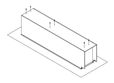
Step 6: Install toe kick panel(G). Fit in the L-shape insert bracket from toe kick panel (G) into side panel (B) bracket and screw the bracket with(3) \( \mathrew{\phi} 3.5 x 14 mm \) screw.
