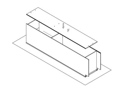
Step 5: Install assembly screws(5) \( \phi 3.5 x 35 mm \) into back panel (D).
