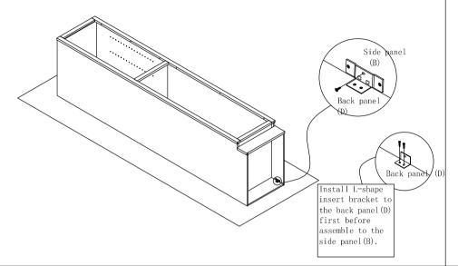
Step 8: Install corner block. Install rainbow bracket to the side panel (B), front frame (A) and back panel (D) with the (4) Ø3.5x16mm screw.
