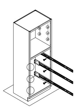
Step 10: Install adjustable shelf(H) and drawer box(I). Put the adjustable shelf on the shelf clips and insert the drawer slide of drawer box to the drawer slide of side panels.
