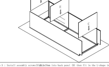
Step 5 : Install assembly screws (5)  $\emptyset$ 3.5x35mm into back panel (D) then fit in the L-shape insert bracket from front frame (A) into bottom panel (C) bracket and screw the bracket with (3)  $\emptyset$ 3.5x14mm screw
